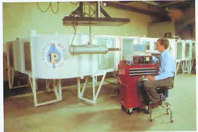
The R & D lab is equipped with a computerized Forward Scattering Spectrometer Probe (FSSP). The FSSP uses precision optics and a laser to measure liquid droplets down to submicron diameters. This FSSP is being inspected before being placed into the wind tunnel.
