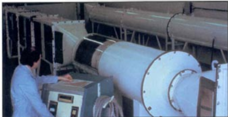
A 30-inch horizontal filter/separators is tested for separation efficiency using the wind tunnel in the R&D lab at Peerless.
