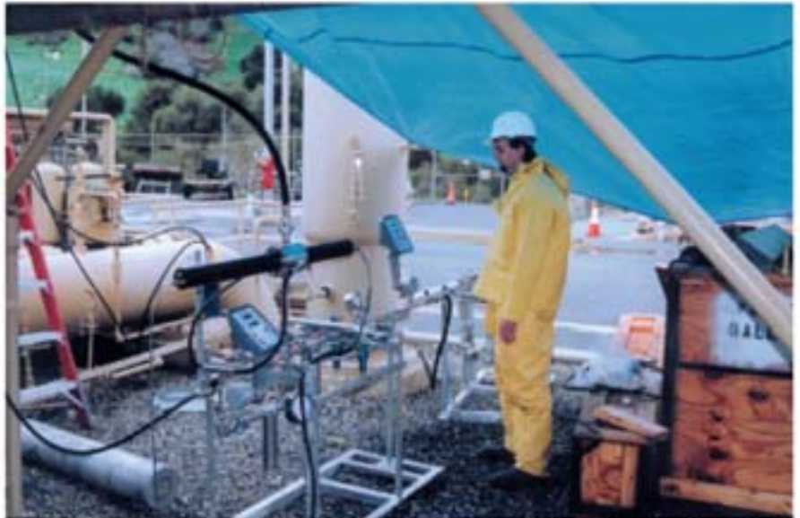
Troubleshoot systems, optimize designs or qualify products with the LISP. Above, a Peerless field engineer utilizes the LISP to count and size pipeline particulates.
